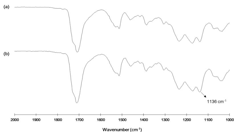
Figure S1. FTIR spectra of PU-A (a) before heating and (b) after heating at 120°C for 10 min.
