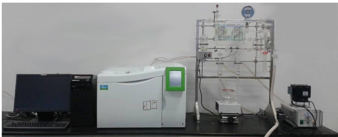
Fig. S9 The photograph of the experimental setup of the photocatalytic H 2 production.
