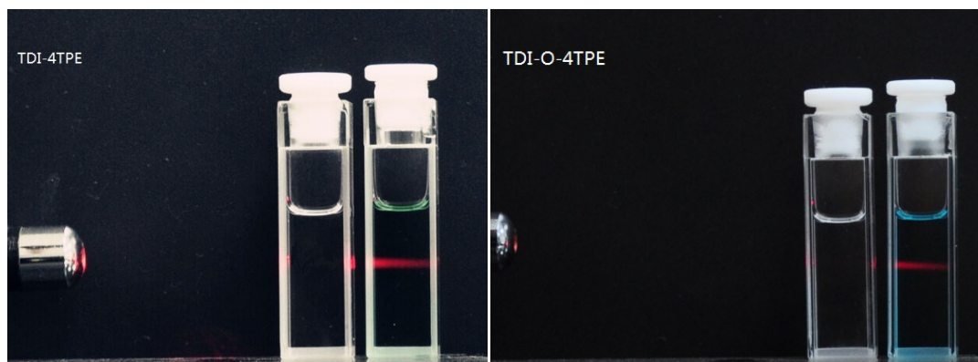
Fig. S7 The demonstrative experiment of Tyndall effect of TDI-4TPE and TDI-O-4TPE in 99% hexane fraction in DCM. The left cuvette in each picture is filled with the solvent without dyes as a blank, while the right one is filled with dyes. A red laser pen passes through the samples from the left. The concentrations of dyes are 1.0 \times 10^{-5} \text{M} .
