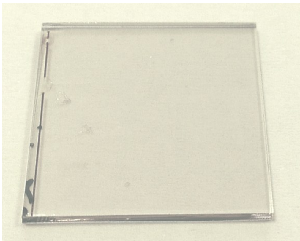
Figure S10. Images of, above, PPCBMB, and below, a PPCBMB thin film (~50 nm) on ITO-glass substrate cast by blade coating from o -xylene.
