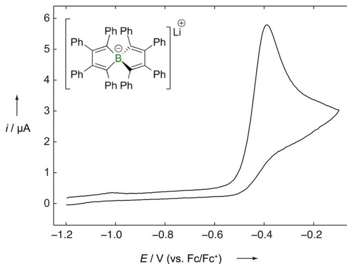
**Figure S1.** Experimental cyclic voltammogram of spiroborate salt **2** measured in thf/0.1 M  $[\text{nBu}_4\text{N}][\text{PF}_6]$  at a scan rate of 250 mV/s. Formal potential:  $E_{\text{pa}} = -0.35$  V.
