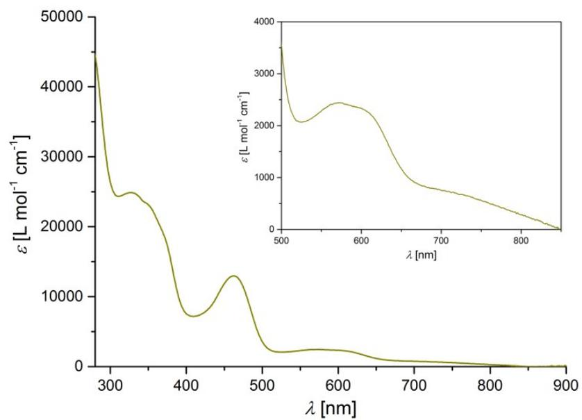
**Figure S2.** UV-vis spectrum of **3** measured in benzene solution (magnified view in the inset).
