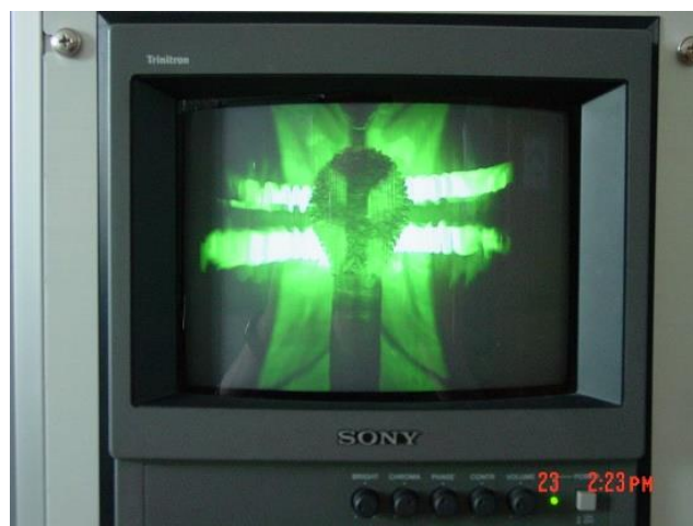
Figure S2: The growth morphology image of the ZnO microrods observed in the FZ furnace.
