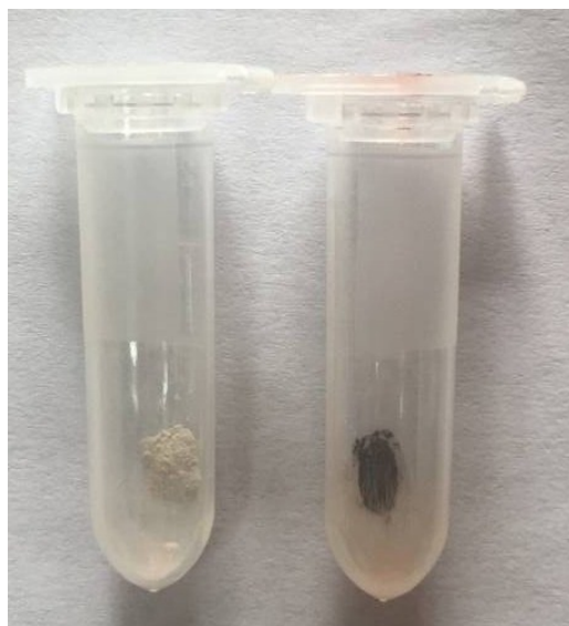
Fig. S4 The colour of the catalysts before and after the reduced reaction
