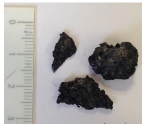
Figure si-3. Picture of slag accumulated at the free surface between LBE and argon cover gas of the sample extraction point in the CRAFT loop.
