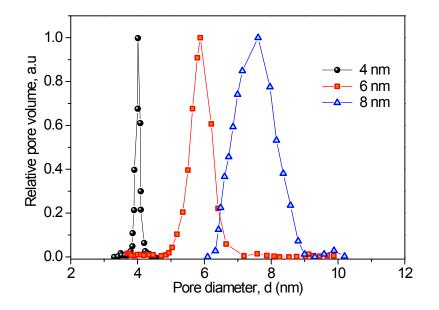
Fig. 1 Pore size distribution obtained from NMR-cryoporometry for the silica mambranes used in or studies.
