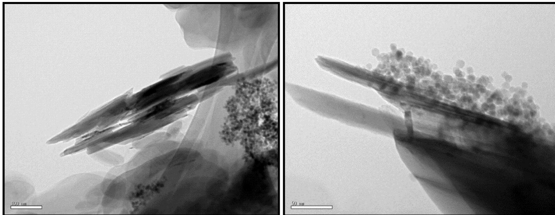
Figure S5. TEM images of h-BN nanoscrolls (BNS) and Fe 3 O 4 NPs hybrids.
