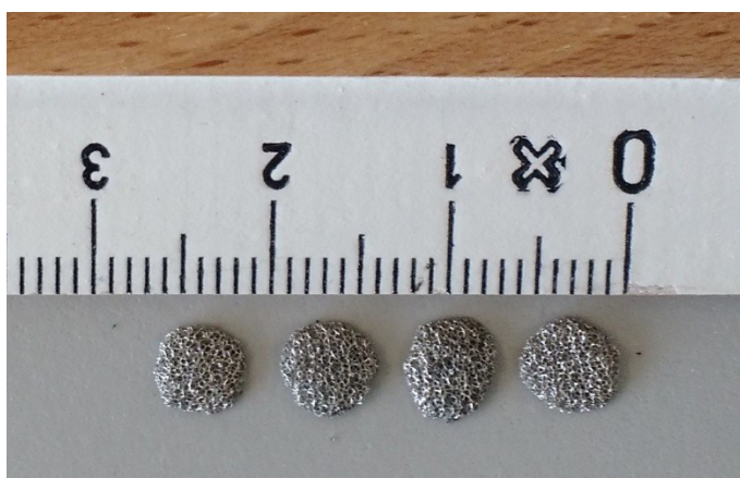
S.Fig. 5: Fresh Ni-Foam pieces loaded in the reactor.
