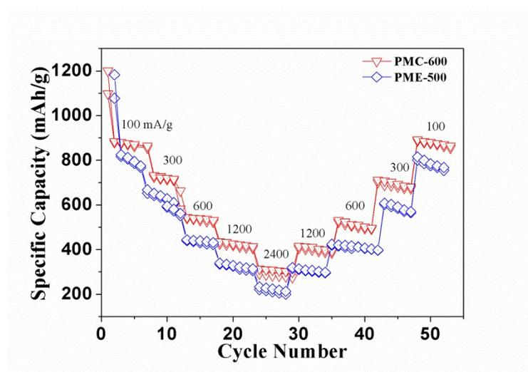
Fig. S6 Rate performance of PMC-500 and PME-500 at different current densities from 100 – 2400 mA · g<sup>-1</sup>.
