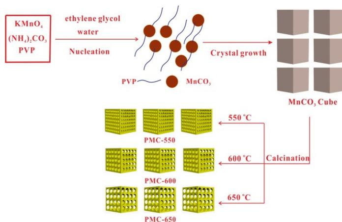
Fig. S5 Proposed growth mechanism for the formation of porous  $\text{Mn}_2\text{O}_3$  microcubes.
