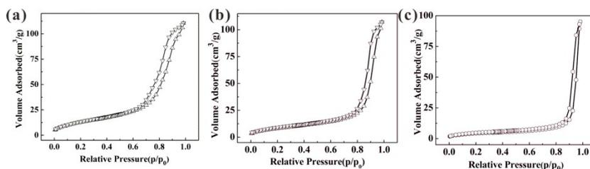
Fig. S4 The  $\text{N}_2$  adsorption-desorption isotherms of  $\text{MnCO}_3$  cube sintered at different temperature for 30 min (a) 550 °C; (b) 600 °C; (c) 650 °C.
