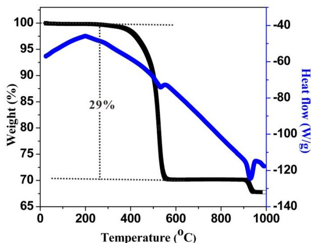
Fig. S3 TGA curves of the as-obtained  $\text{MnCO}_3$  microcubes.
