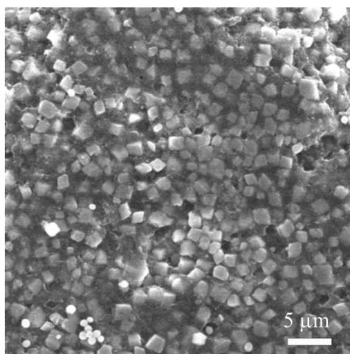
Fig. S7 SEM image of PMC-500 electrode after 50 discharge-charge cycles.
