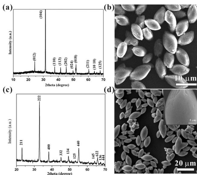
Fig. S2 (a-b) the XRD pattern and SEM images of  $\text{MnCO}_3$  micro-ellipsoid prepared in absence of PVP; (c) XRD pattern and SEM image of  $\text{MnCO}_3$  micro-ellipsoid calcined at 500 °C for 30 min (PME-500).
