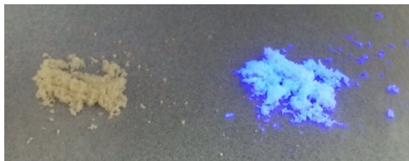
Fig. S23. Photograph of powder of selenophene-1,1-dioxide 5 (left) and thiophene-1,1-dioxide 3 (right) upon irradiation of 254 nm light. Due to instability of the compound of 5 the powder was slightly colored.
