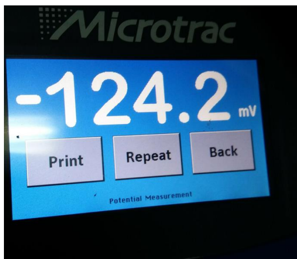
Figure S6. Optical images of the zeta potential of \text{Fe}_3\text{O}_4@\text{SiO}_2 nanopindles in ultrapure water.
