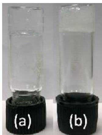
Figure S6 Gels prepared by dissolving gelators in DMSO, EtOH and H 2 O in different ratio (a) DMSO:H 2 O (1:2) at 0.5 mg/ 0.5 ml (b) EtOH:H 2 O (1:2) at 0.8 mg/0.5 ml
