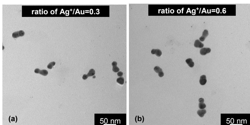
**Fig. S3.** TEM images of the bimetallic nanostructure with *p*-MBA sandwiched between the two metals with Ag<sup>+</sup>/Au molar ratios ( $R_{Ag^+/Au}$ ) of 0.3 (left) and 0.6 (right) related to Figure 6 in the text.
