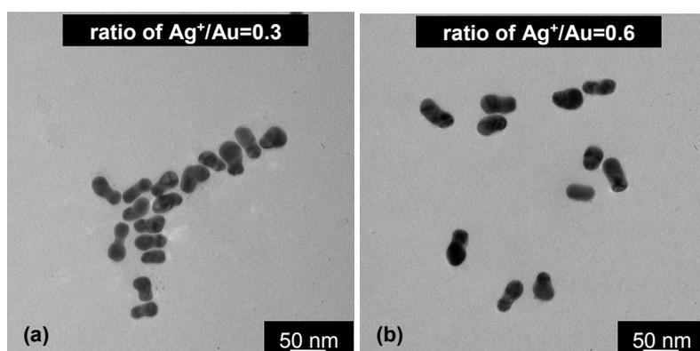
**Fig. S1.** TEM images of the gold dimers after the deposition of silver at the  $\text{Ag}^+/\text{Au}$  molar ratios ( $R_{\text{Ag}^+/\text{Au}}$ ) of 0.3 (left) and 0.6 (right).
