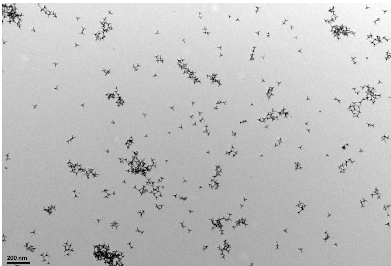
Figure S1. A large scale view of a low resolution TEM image of as-synthesized PbSe seeded PbS tetrapods. From typical sample sizes of \sim 500 particles, we deduced that the yield of tetrapods for this synthetic strategy generally ranged from 90-95 % on average.
