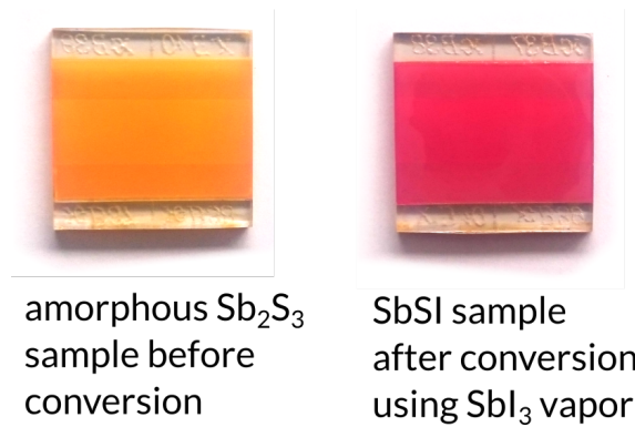
Fig. 1 Photograph of an amorphous \text{Sb}_2\text{S}_3 sample and a SbSI sample after conversion with \text{SbI}_3 and rinsing in ethanol.
