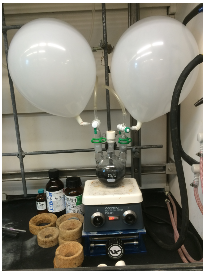
Figure S2. Equipment set up and appearance of debenzoylation reaction on 10 g scale of tetra-benzyl-di- O -acetyl gluco septanose.
