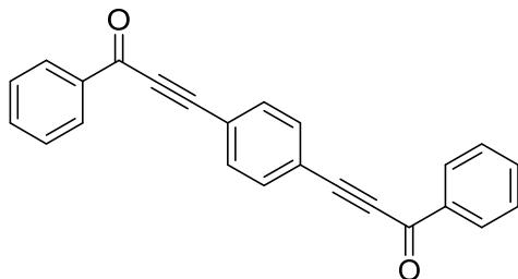
In deviation from the general procedure, 1.00 equiv of 1,4-diiodobenzene were used as aryl iodide **1** while the amount of all other reactants was doubled. With benzoyl chloride as aryl chloride component, 199 mg (0.595 mmol, 60%) of **4k** were obtained as a yellow solid. Purification was performed using the flash purification system (*n*-hexane/DCM 4:1 → 1:1 → 0:1), Mp 185 °C (lit.<sup>4</sup> 191 °C).
