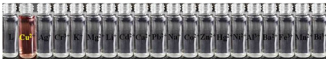
Fig. S5: A color change photograph for \text{Cu}^{2+} and the other metal ions under visible light.
