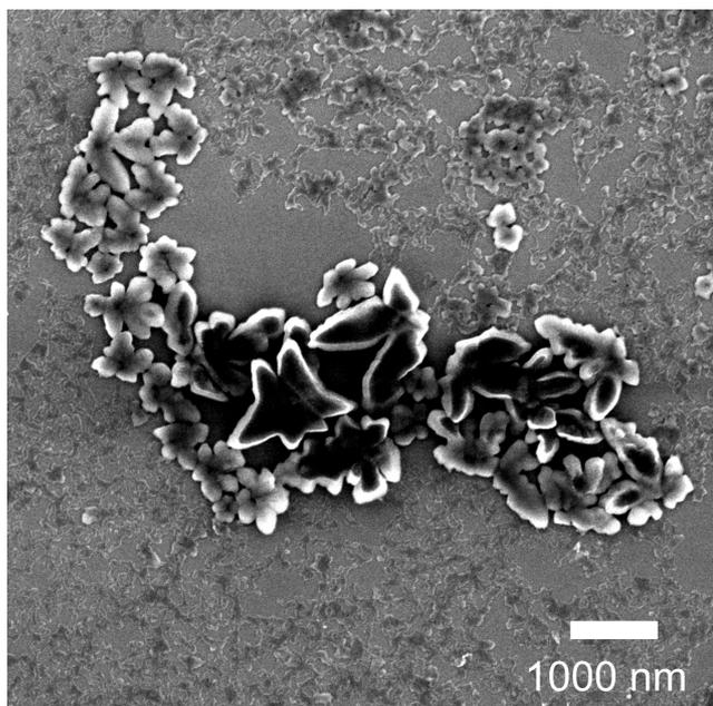
**Figure S4.** SEM image of a  $C_{60}$  film when depositing 250  $\mu\text{L}$   $\text{CHCl}_3 / C_{60}$  solution at  $P=500$  mbar on an area of  $3.5 \text{ cm}^2$ . For volumes over  $\sim 200 \mu\text{L}$ , overgrowth of large  $C_{60}$  crystals occurs.
