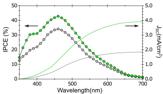
**Figure S11.** Internal photon-to-current conversion efficiency (IPCE) measurements and corresponding  $J_{sc}$ . grey: F-C<sub>60</sub>, green: 2 layers S-C<sub>60</sub> on F-C<sub>60</sub>.
