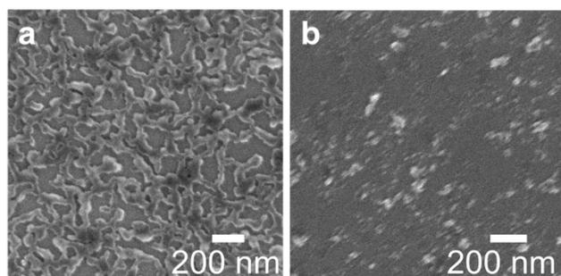
**Figure S5.** Solubility of  $C_{60}$  films deposited on Si without light-induced polymerization. SEM images (a) Pristine  $C_{60}$  film; (b) film residues after chloroform rinsing without prior light exposure.
