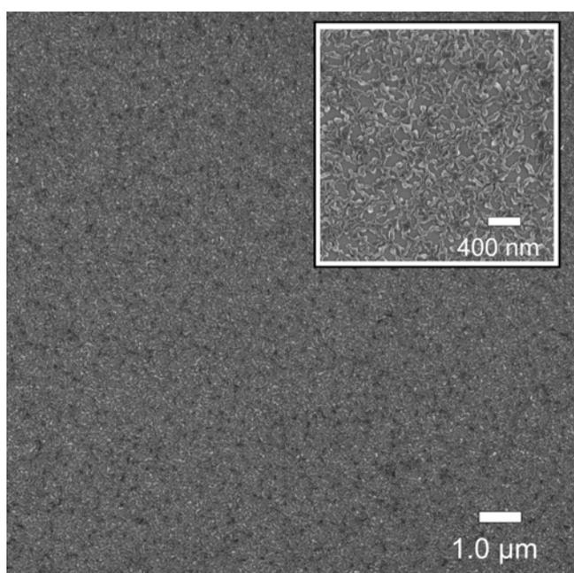
**Figure S1.** Large scale SEM image of a nanostructured  $C_{60}$  film and magnification (inset).
