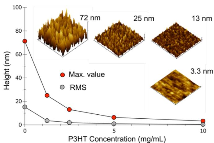
**Figure S6.** Infiltration of stabilized  $C_{60}$  nanostructures with P3HT. P3HT films were coated at 1000 rpm for 30 s from chloroform solutions. Red: maximum peak-to-valley
