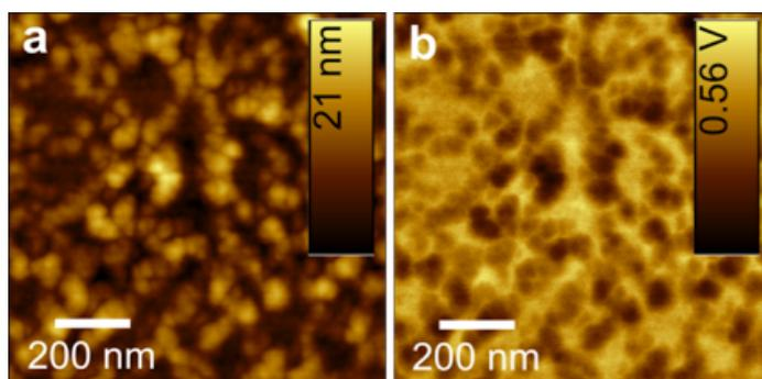
**Figure S7.** Scanning force microscopy images of nanostructured  $C_{60}$ , after light exposure and partial P3HT coating (2.5 mg/mL, 1000 rpm). (a) SFM topography showing reduced height difference and filling of the voids in the  $C_{60}$  layers, as well as the stability of the  $C_{60}$  domains; (b) Electrostatic force microscopy phase showing  $C_{60}$  domains (dark) and P3HT filling (bright).
