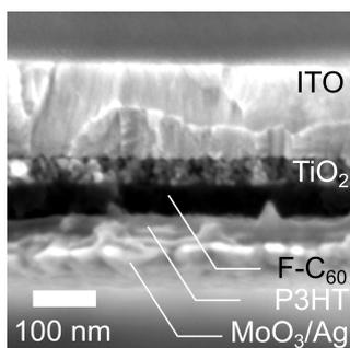
**Figure S9.** SEM cross-section image of a light-stabilized planar bilayer  $C_{60}$ /P3HT solar cell.
