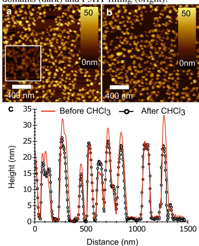
**Figure S8.** Evolution of the morphology upon film drying and consecutive film stabilization. (a) SFM image of a nano-structured  $C_{60}$  film after drying for 6 h at  $80^{\circ}\text{C}$  under nitrogen atmosphere and photo-polymerization, the inset shows the pristine film; (b) SFM image of the same area as (a) after solvent rinsing; (c) representative profiles extracted from (a) and (b).
