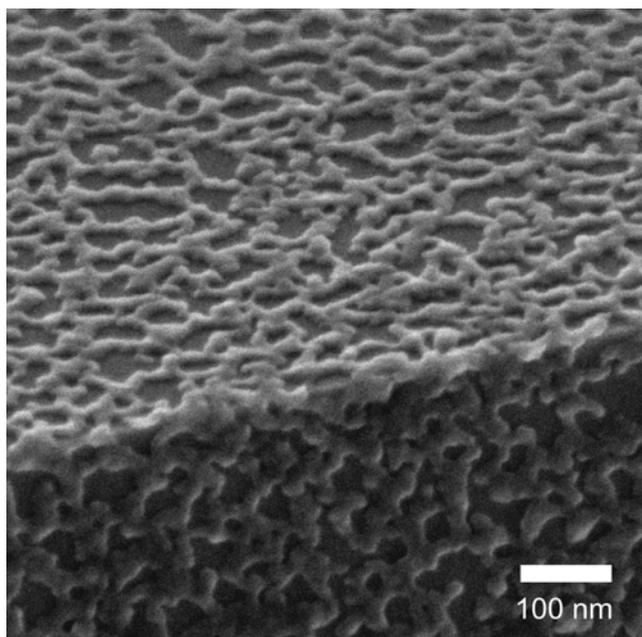
**Figure S2.** Flexibility of a C<sub>60</sub> nanostructured thin film demonstrated by imaging over perpendicular surfaces of a silicon substrate.
