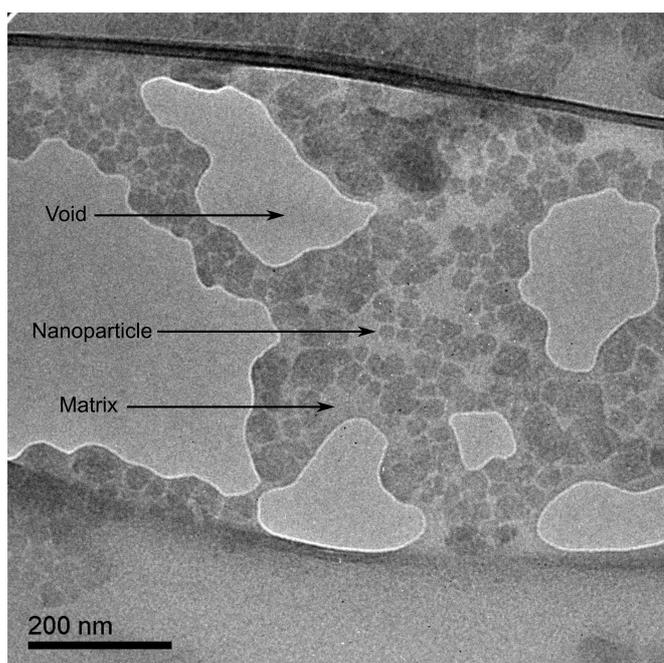
**Figure S3.** TEM image of a nanostructured C<sub>60</sub> film. The image shows 10-50 nm large C<sub>60</sub> particles embedded in a C<sub>60</sub> matrix.
