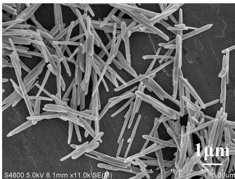
Fig. S1 FE-SEM images of pure \text{Bi}(\text{OHC}_2\text{O}_4)\cdot 2\text{H}_2\text{O} .
