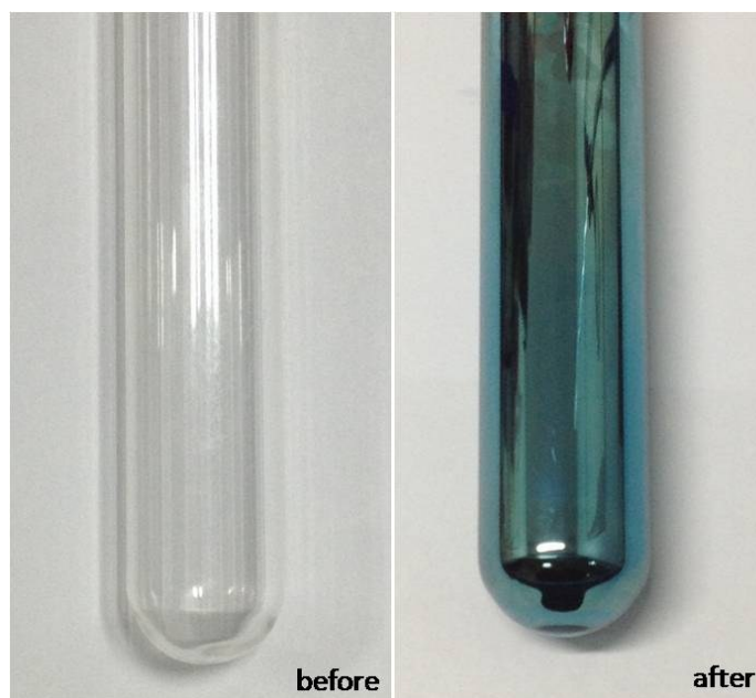
Fig. S4 Photograph of the test tube for reduction of silver-dodecylamine complexes by acetaldehyde in toluene.
