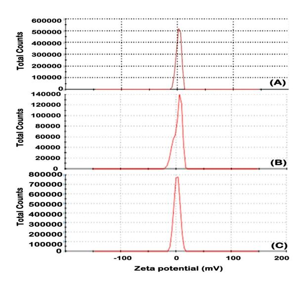
**Supplementary Figure 1.** Zeta particle size distribution peaks: **A)** Chitosan nanoparticles, **B)** *Gymnema sylvestre* leaf extracts derived biomolecule-loaded chitosan nanoparticles (GSCZNPs) and **C)** *Cinnamomum zeylanicum* bark extracts derived biomolecule-loaded chitosan nanoparticles (CZCNPs).
