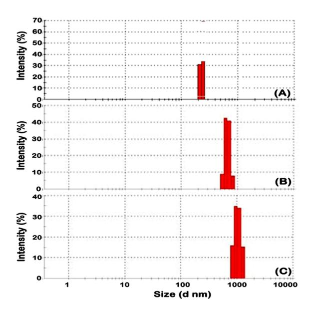
**Supplementary Figure 2.** Results of Particle Density Index: **A)** Chitosan nanoparticles, **B)** *Gymnema sylvestre* leaf extracts derived biomolecule-loaded chitosan nanoparticles (GSCZNPs) and **C)** *Cinnamomum zeylanicum* bark extracts derived biomolecule-loaded chitosan nanoparticles (CZCNPs).
