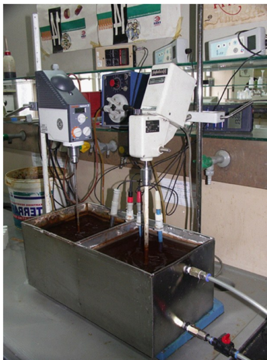
Figure S1. Continuous flow reactor for \text{Fe}_3\text{O}_4 and ferrite nanoparticles production.
