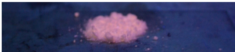
Figure S4. The digital photos of the prepared CDs-TbEu 0.2 composites in solid states under the UV light (365 nm).
