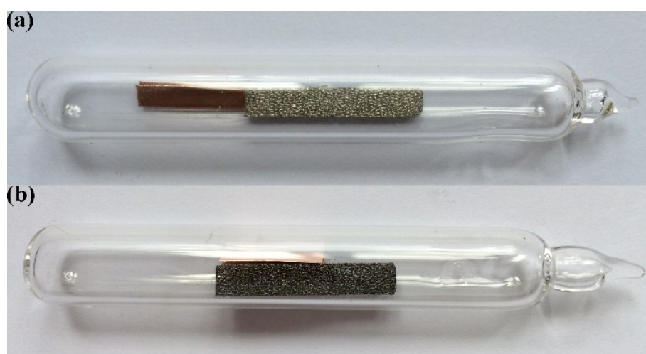
Fig. S1 Photograph of the sealed quartz tube with PMMA/Cu film and Ni foam. (a) before
