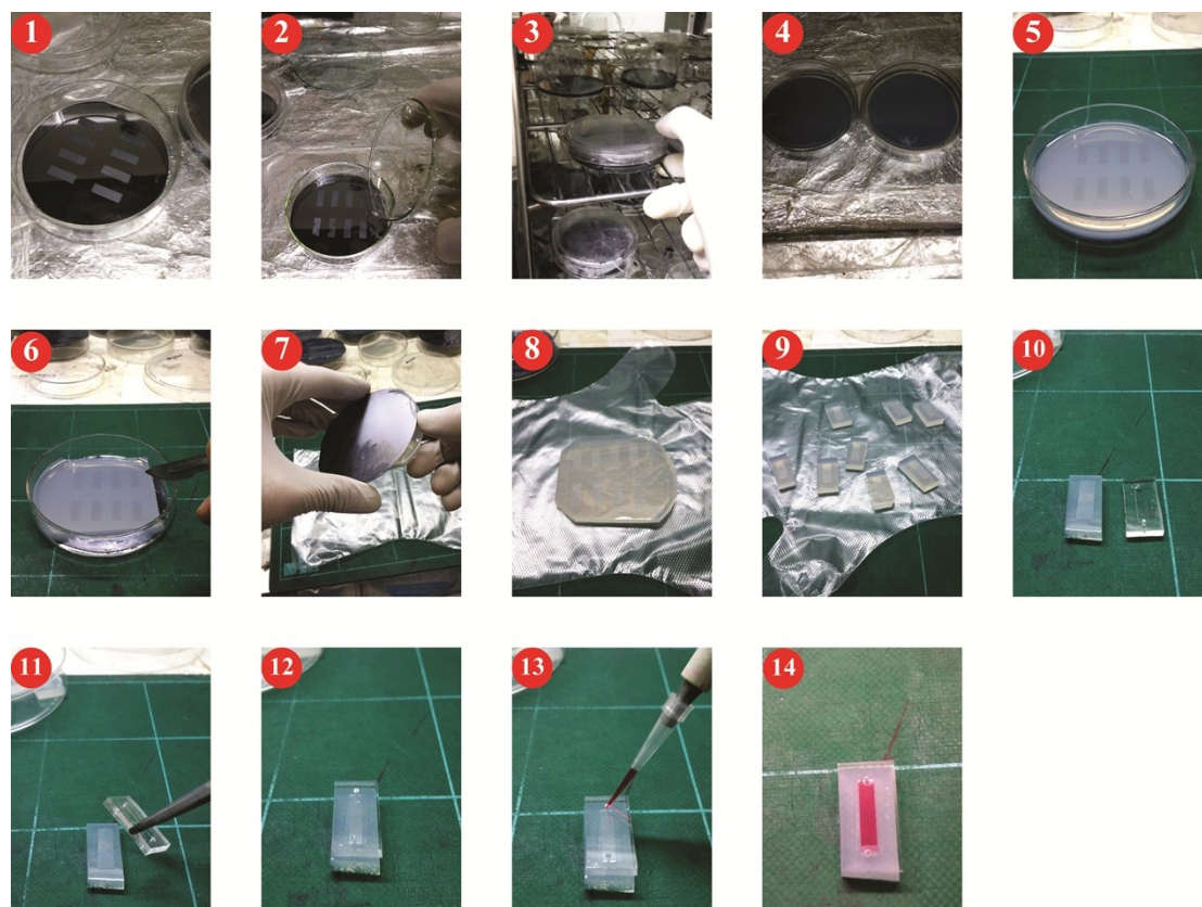
Fig. S1 Fabrication of agarose microwell array. 1. The SU-8 templates was formed on the silicon wafer as standard lithography protocol and placed in a glass dish. 2. Boiled agarose solution was poured into the dish containing wafer. 3. Place the cast to 65°C incubator and preserve for 30 min. 4. Cooling down the cast at room temperature for 3h. 5. Gelation of agarose gel on SU-8 mold. 6. Cut the casting complex out from dish by surgeon knife. 7. Peel the gel from silicon wafer base. 8&9. Cut the gel into uniform pieces. 10-12. Assemble the PDMS-agarose chip by physically attaching PDMS channel to the gel surface. 13. Sampling by direct pipette transfer.
