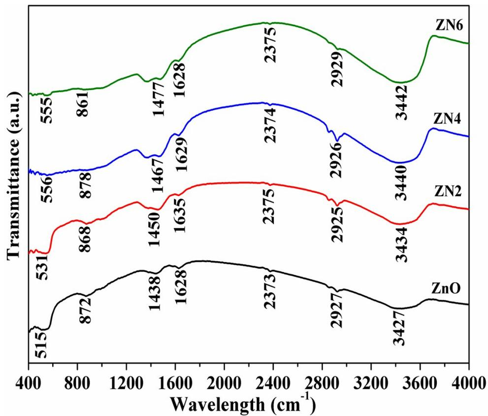
Fig. S1 FTIR spectra of undoped and Ni-doped ZnO NPs
