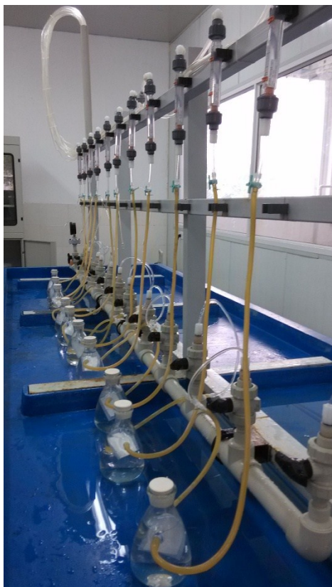
Figure S1. The flow-through adsorption test in lab-scale simulated seawater adsorption system
