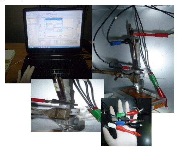
**SM-Fig.1.** Electrochemical Impedance Spectroscopy (EIS) system used in this study with three electrodes; (i) a PGE, (ii) a Ag/AgCl/ 3M KCl reference electrode and (iii) a platinum wire as the auxiliary electrode. A typical test result recorded on the computer (upper left).
