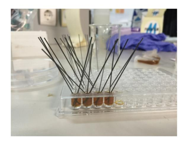
**SM-Fig.2.** Deposition of GNRs onto the PGE surface by simple incubation.
