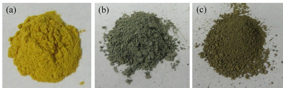
Fig. S2 The digital photos of natrojarosite (a) before adsorption; (b) after adsorption; (c) washed by distilled water under ultrasonic after adsorption
