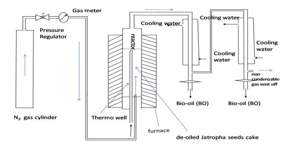
Supporting Fig 1: Schematic representation of experimental set-up for pyrolysis of deoiled jatropha seeds cake.
