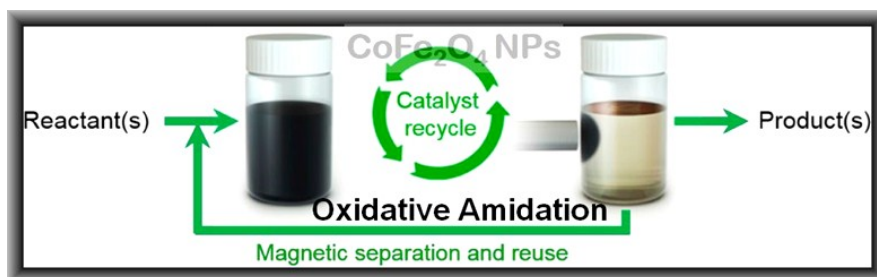
Separation of the catalyst from the reaction mixture by an external magnet.
