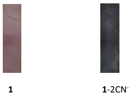
Fig. S9 Color change of 1 -based test strips before and after addition of \text{CN}^- .
