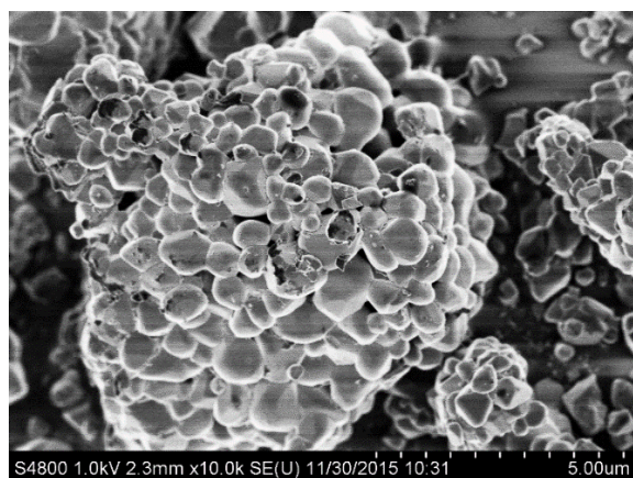
Fig. S4 SEM image of as-prepared LMO sample.
