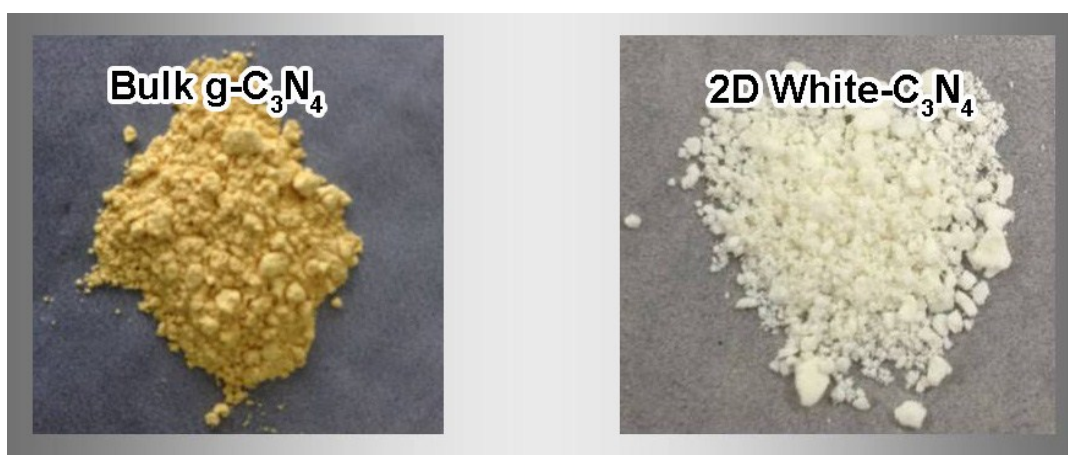
Figure S2. Photographs of the bulk g\text{-C}_3\text{N}_4 and 2D White- \text{C}_3\text{N}_4 .
