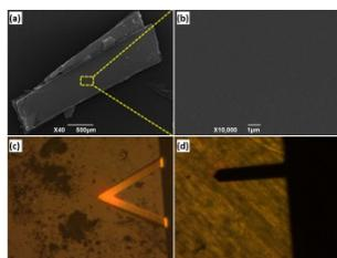
**Fig. S1.** The pristine surface state of biotite sample under electron microscope and AFM loading sample platform, of which (a) the SEM image of biotite sheet, (b) the biotite (001) surface, (c) the probe NP-S10 within contact mode, and (d) the probe MESP within tapping mode.
