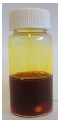
Figure S 1. Photograph of 30 wt% P3HT composite in THF (total polymer concentration of 3 wt%).
