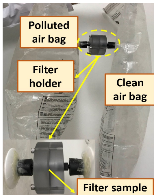
Figure S1. Digital picture of the air filtration experimental setup
