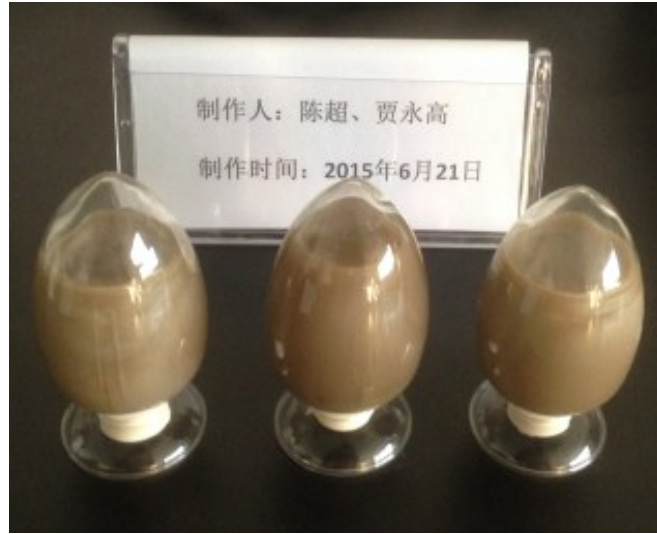
Fig. S5 Photograph of AgNW inks left still at room temperature for 6 months where C_{\text{AgNW}} , C_{\text{PVP}} and V_{\text{NMP}}/V_{\text{EG}}/V_{\text{glycerol}} were kept as 5 mg/mL, 30 mg/mL and 4:5:1.
