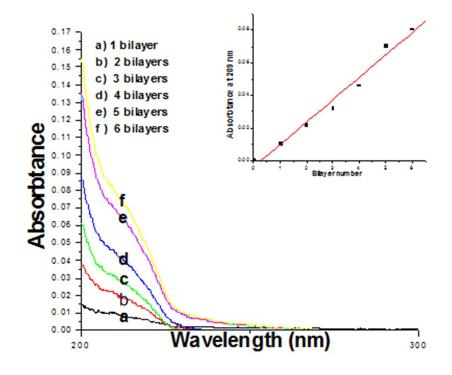
Figure S1. UV-Vis spectra of different PS-PAA/PAH multilayers with different deposition cycles on glass slides. The inset image was that the absorbed value at 209 nm vs the desposition cycles.
