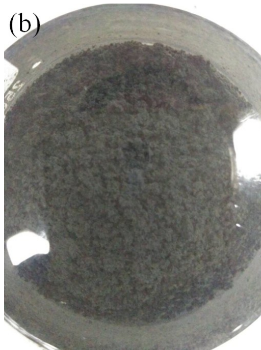
Fig. S 2. The sludge morphologies conditioned by (a) CPTA and (b) TPTA.
