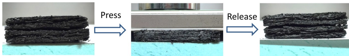
Figure S1. Digital photos of 3DGFs-30 showing the compressing and releasing process.
