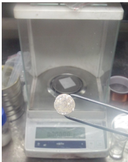
Figure S2. The sodium anode after 100 cycles at the current density of 100 \text{ mA g}^{-1} with a cut-off capacity of 500 \text{ mA h g}^{-1} .
