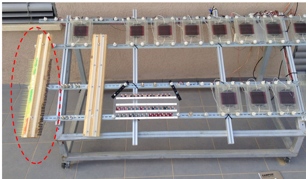
Fig. S1. Photograph of the setup used for outdoor aging studies. The EPR tubes with the polymer films inside are highlighted with a dashed red line.
