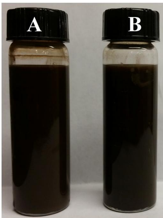
Figure S3. 4 \text{ g L}^{-1} \text{MnO}_2 suspensions, containing 0.2 \text{ g L}^{-1} of (A) PCA and (B) PHA 3 days after ultrasonication
