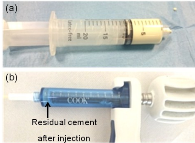
ESI. 5. a) The mixture of Spine-Ghost cement with water ( L/P = 0.4 \text{ mL/g} ) in the syringe before injection, b) the residual amount of Spine-Ghost cement in the DUROJECT syringe after injection (about 0.5 mL).
