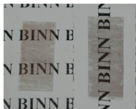
Fig. S8 the photographs before (left side) and after (right side) bend test of the CuS/PET, Cu nanotrough/PET and CuS nanotrough/PET electrode.
