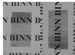
Fig. S8 the photographs before (left side) and after (right side) bend test of the CuS/PET, Cu nanotrough/PET and CuS nanotrough/PET electrode.
